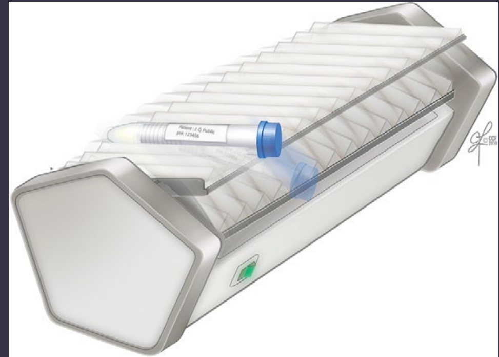
Mixing of the semen sample and TEST-yolk on a test tube rocker for 5 min
